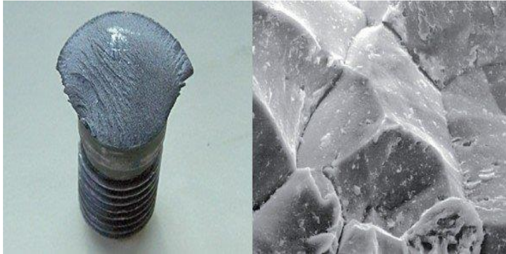
Figure 1.8 Cracks due to the hydrogen embrittlement [61].
