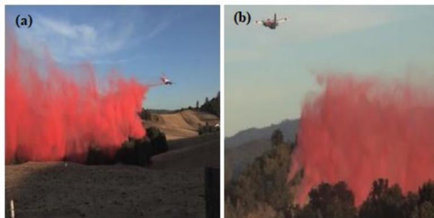
Figure 7.14 An aircraft fire-tanker is discharging red fire extinguisher liquid [80].
