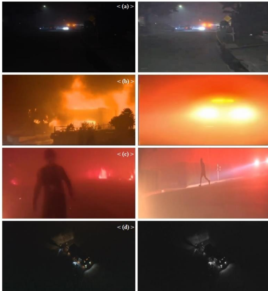
Figure 2.6 Challenges of night-time fire detection a) A dark image with a low contrast against the background (left) and the same image manually enhanced by changing color curves.; b) Images with insufficient texture.; c) Noisy night-time images.; d) An aerial image of a vehicle and the corresponding black-white image.
