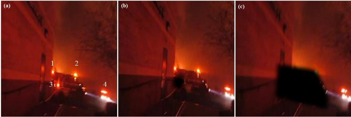
Figure 7.10 A misclassification of a non-fire scene as fire due to flashing headlights [76]. An originally misclassified video in (a) with headlights 1, 2, and 3 flashing while 4 non-flashing. Flashing headlight 3 is blacked out with mask M1 in (b); however, the prediction is still fire. Vehicles with all flashing headlights are masked out with mask M2, and non-flashing headlight 4 of another vehicle is preserved as it is in (c). Now, the prediction changed from fire to correctly non-fire.
