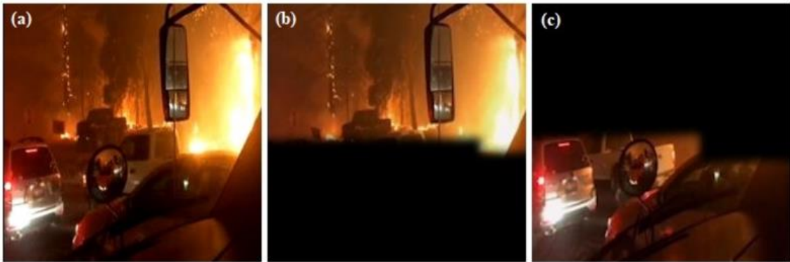
Figure 7.9 A misclassification of a fire scene as non-fire due to headlights [75]. An originally misclassified video in (a). When vehicles with headlights are blacked out with mask M1 in (b), the video is correctly classified as fire. When all fire objects are blacked out with mask M2 in (c), then the decision is non-fire.
