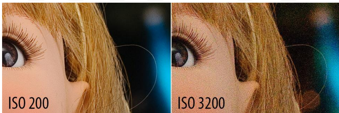
Figure 2.4 Noise contributed by large ISO [84]. High ISO values also magnifies the noise (right) while enhancing the image (left). Thus, it should be used cautiously.
