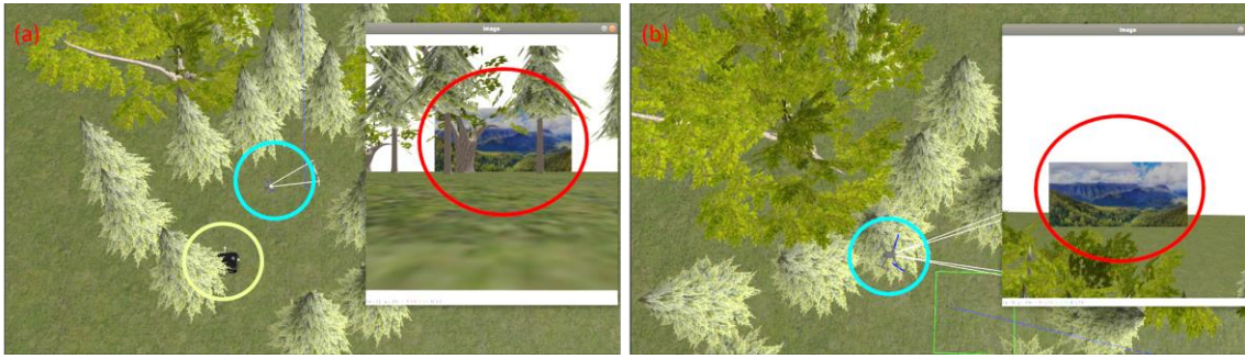
Figure 4.5 UAV taking off to a predefined altitude and scanning environment. Left (a) take off, right (b) scanning. Red circle: UAV front-looking camera footage; blue circle: UAV; yellow circle: UGV.
