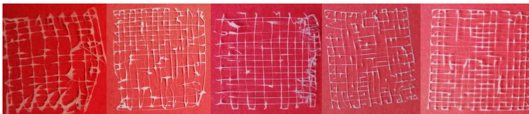
Figure 3.13 Printability of PCL_DCM and PCL_CF scaffolds at speeds above 5 mm/s with 480 kPa.
