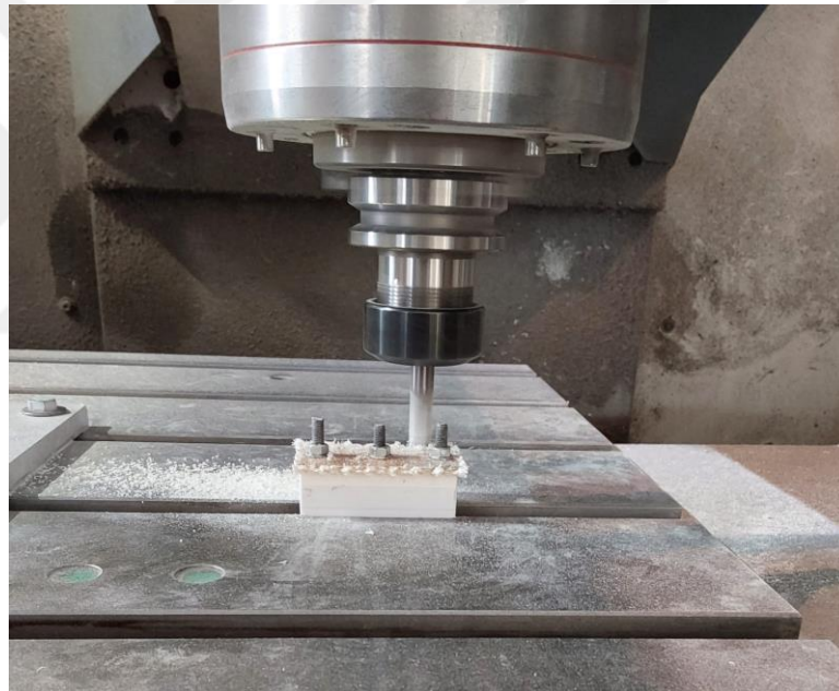
Figure 5.6 Machining of a) BFRP and b) S2-GFRP samples
