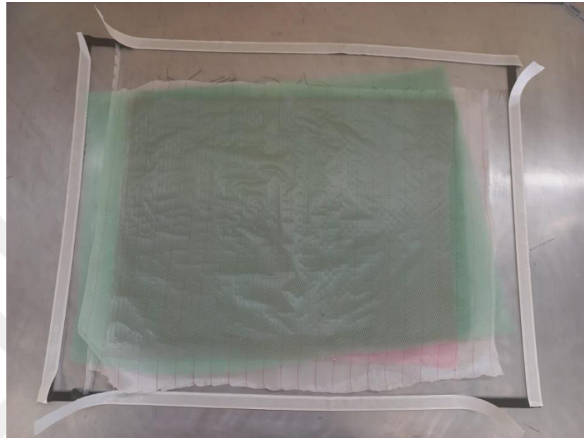
Figure 2.1 Assembly before the vacuum bag
