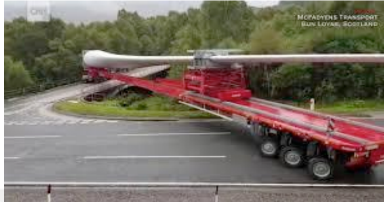
Figure 2. 9 One example of the difficulties experienced in turbine blade transportation. ( https://www.youtube.com/watch?v=rxvuMv2MED0 )
