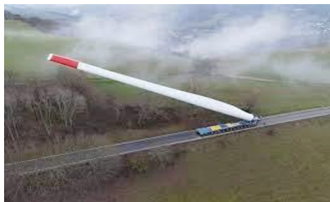
Figure 2. 7 An example of turbine blade transport ( https://www.reddit.com/r/EngineeringPorn/comments/knp_ejd/67metre_wind_blade_being_transportated_by_road/?rdt=53185 )
