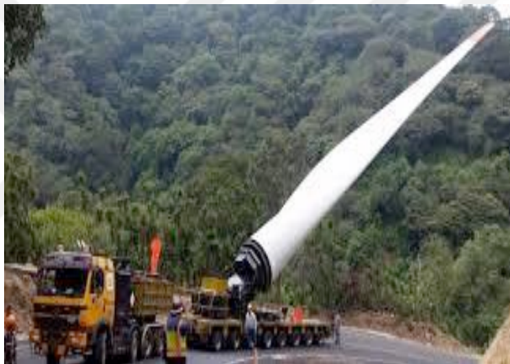
Figure 2. 8 Example of turbine blade transport ( https://www.craneblogger.com/featured-articles/goldhofer-ftv-300-blade-transport-device-moves-wind-turbines-up-tough-terrain/2016/09/02/ )
