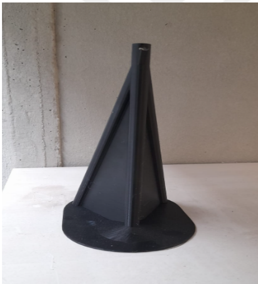
Figure 3. 10 3D printed wind turbine tower structure with three legs and a curtain wall system between the legs
