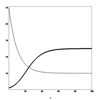
Figure 2. Stabilization of the stored energy W(t) (solid line) under the control field u(t) (thin dot line) at the level  $W_*=25$ .
