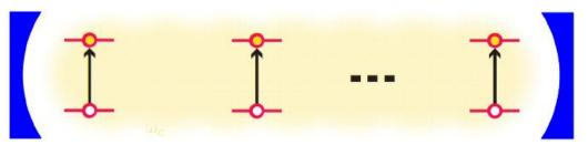
Figure 1.Schematic representation of a globally charging Dicke battery: many twolewel quantum systems are coupled to the same cavity; Fig. based on [1].
