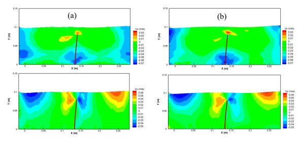
**Figure 15.** Comparison between velocity contours of (**a**) the  $\delta$ -SPH scheme and (**b**) the standard SPH at t = 1.44 s.
