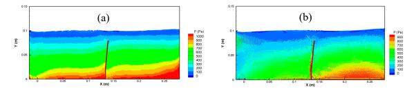
**Figure 14.** Comparison between free-surface profiles of (**a**) the  $\delta$ -SPH scheme and (**b**) the standard SPH at t = 1.44 s.
