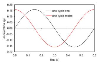
Figure 4. Idealized pulses to represent near-fault ground motion.
