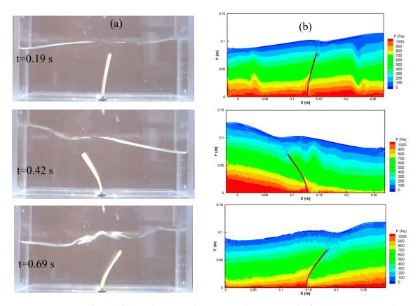
**Figure 7.** Free surface profiles under one-cycle cosine acceleration impulse for (**a**) experiment and (**b**) simulation.
