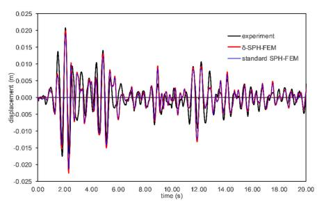
Figure 11. Horizontal tip displacement of the elastic plate.
