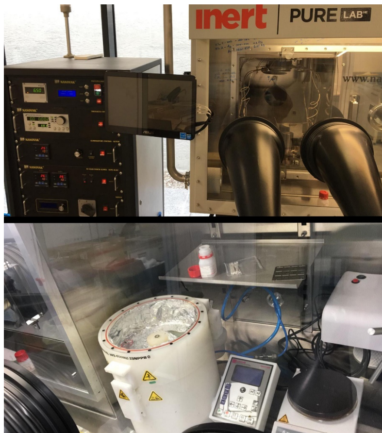
Figure. 3.8.3 The thermal evaporation system integrated to the inert glove box
