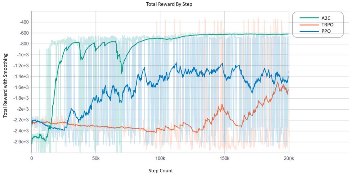
Figure 13. Total reward with smoothing gained by step for each algorithm
