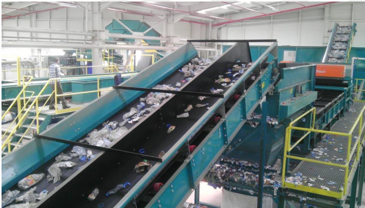
Figure 3. 9 Plastic sorting and cleaning process
