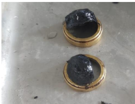
Figure 4. 1 Softening point test, the bitumen separated from the ring wall by rupture
