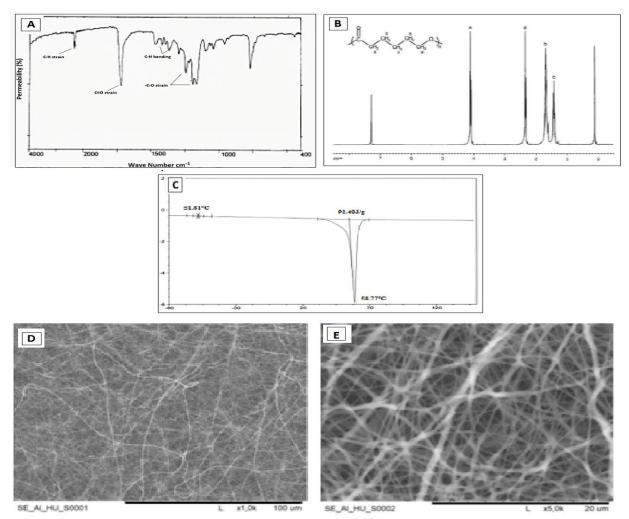
Figure 2. (A) FTIR spectra of  $\varepsilon$ -PCL scaffolds at approximately 40.000 to 400 cm<sup>-1</sup> indicated by black lines, (B) H-NMR spectrum of  $\varepsilon$ -PCL, (C) DSC thermogram of  $\varepsilon$ -PCL, SEM images of micropores and macro channels of  $\varepsilon$ -PCL (D; X1000), (E; X5000)
