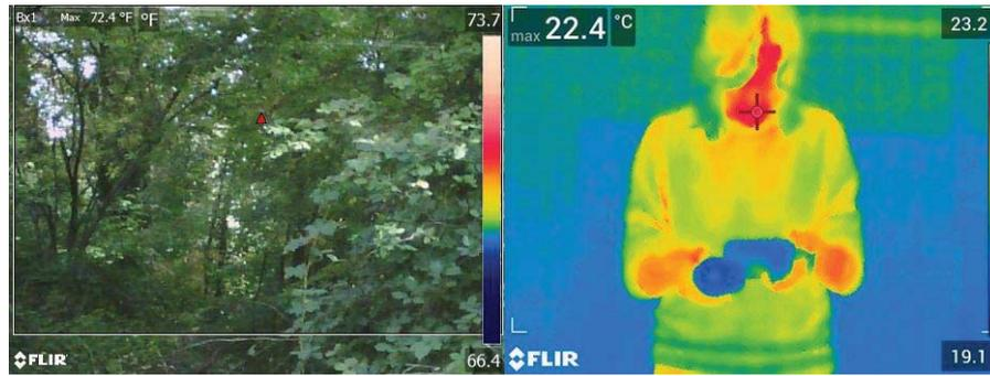
**Figure 2.5 Thermal reflection from glass**
