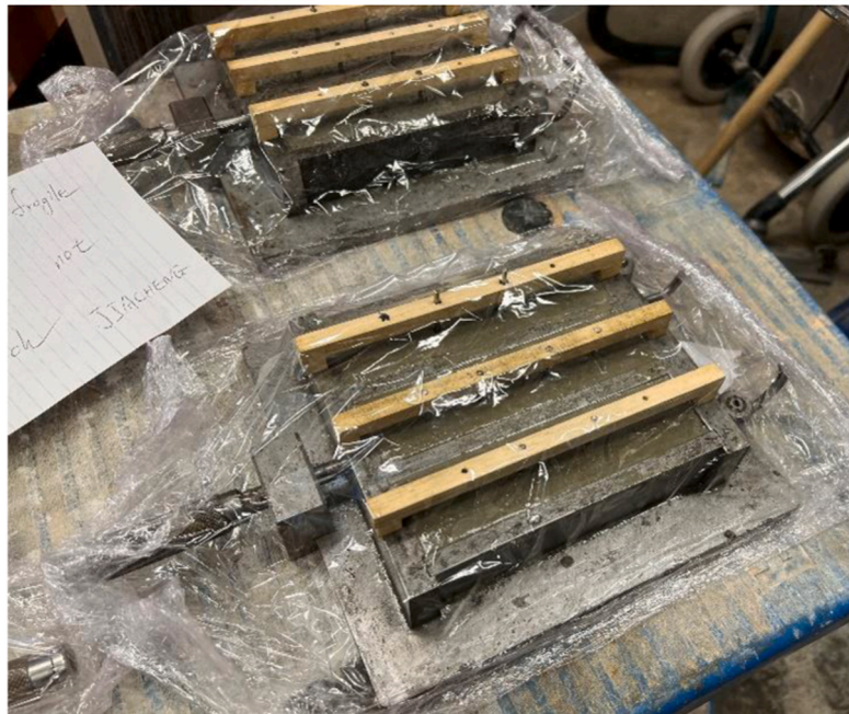
Fig. 1. Fabrication of samples: (a) electrode configuration and dimension of prismatic samples at front, top, and side views, unit in mm (b) fresh sample in the mould sealed with PVC film.
