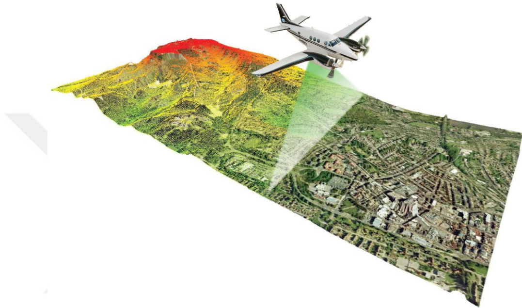
Figure 1.1.2 LIDAR land-scanning system is incorporated on a airplane is using to obtain land surface with high resolution [22].
