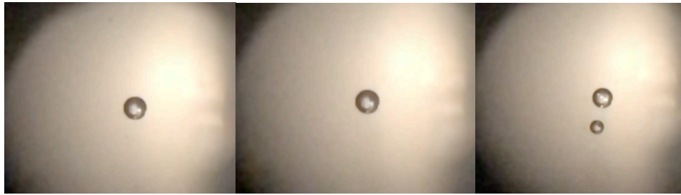
Figure 4.1.2 Bubbles that are created with different laser energy levels are shown. Bubble in the left image created with 1mJ laser energy. Bubble in the middle image created with 1.2 mJ laser energy and bubbles in the right image created with 1.5 mJ. It can be seen that couple of bubbles appeared when laser energy increased.
