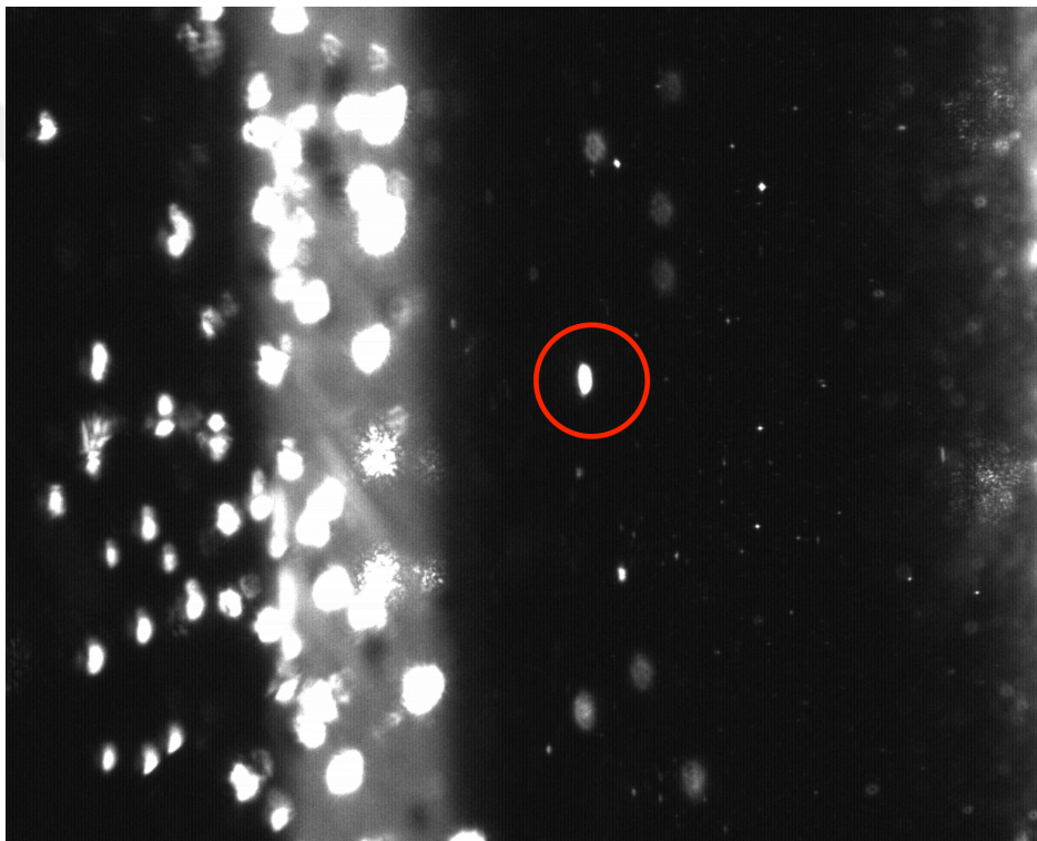
Figure 3.2.1.1 A sample image that was taken with the CCD camera. Fluid enlightened by the slit light to let bubbles glow. Glowing bubble is encircled with a red circle.
