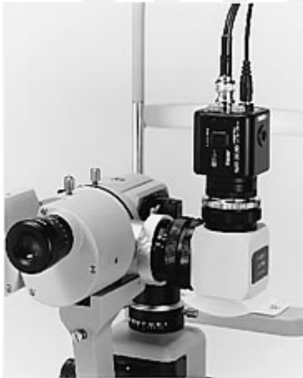
Figure 3.1.2.1 Beam splitters can be attached in front of the eyepieces and provide one extra mount for attaching digital camera to the laser system.
