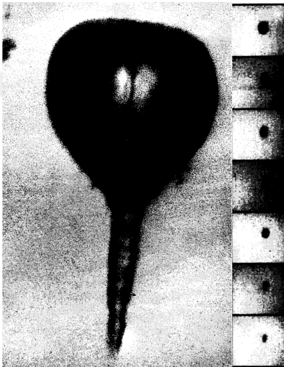
Figure 2.2.1.1 Jet flow is showed on left. It forms with the collapse of the bubble. Bubble collapse is showed in serial images on the right side of the image.
