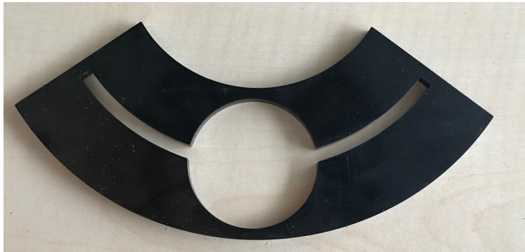
Figure 3.1.2.3 Arc is created with a CNC system.
