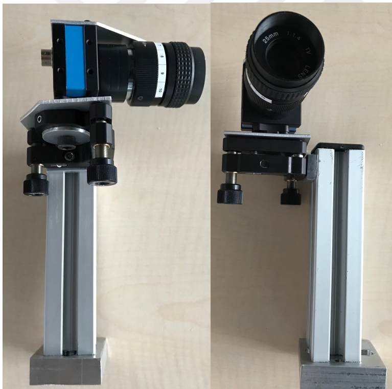
Figure 3.1.3.1 CCD camera and its metallic footing is shown from two different angles.
