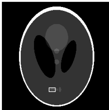
Figure 3.3.2.4.1 The illustration of the targeted region to investigate CNR values from reconstructed images by the proposed method.
