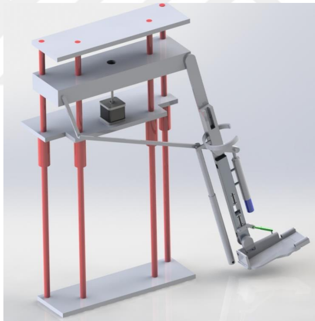
Figure 3.2.3.4 Conceptual design of test bed a) Test bed with cam b) Test bed with ballscrew
