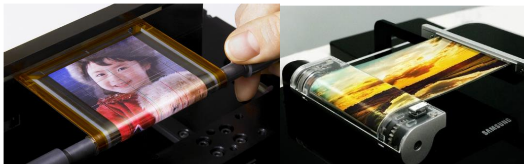
Figure 1.1.2 Rollable OTFT used OLED displays manufactured by Sony and Samsung.
