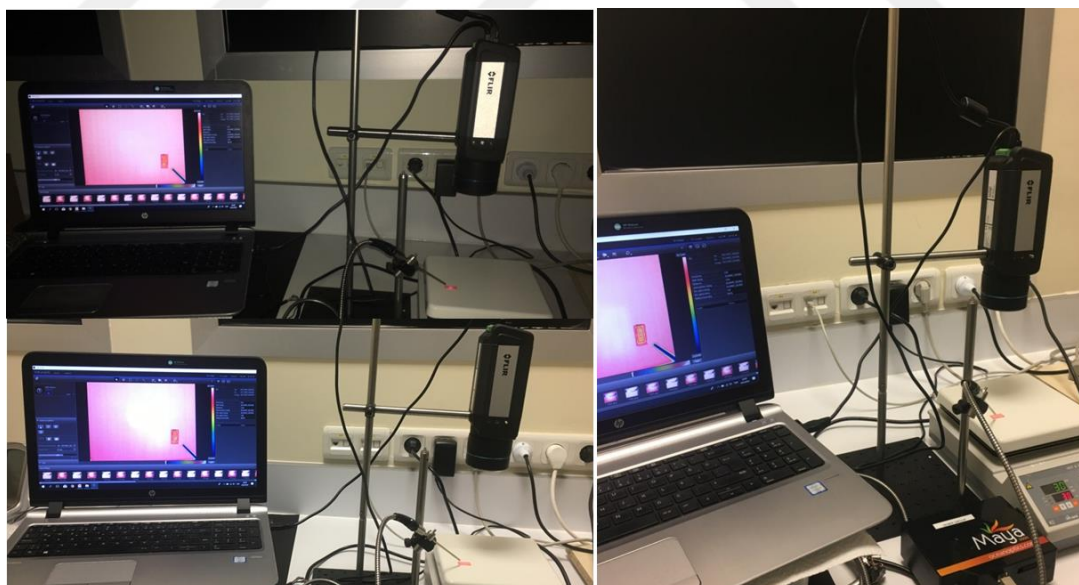
Figure 7.2. 11 Thermal test measurement setup photographs for film form of the samples. Reprinted with permission from [117]. Copyright 2019 WILEY-VCH Verlag GmbH & Co. KGaA, Weinheim.
