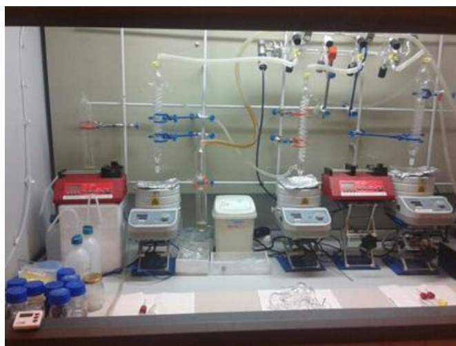
Figure 2.1.2. 1 Nanocrystal synthesis system composes of shlenk-line, heater, vacuum pump, vacuum gauge, condenser, clips and temperature probe.
