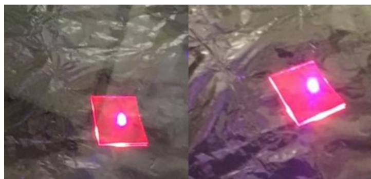
Figure 7.2. 15 The photograph of spin-coated and sealed HI shell NPL film samples (a) and (c) without UV illumination, (b) and (d) under UV illumination. Reprinted with permission from [117]. Copyright 2019 WILEY-VCH Verlag GmbH & Co. KGaA, Weinheim.
